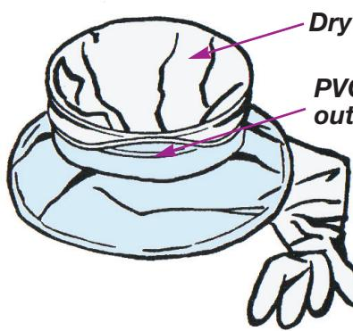
**Step 3.** Insert the Dry Box Glove (with thumb pointing up) through the PVC Glove Extension, leaving enough of the cuff to fold over the PVC Ring outline.
