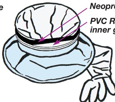
**Step 4.** Place the Neoprene Band over the PVC Ring outline so that it fits within the groove of the PVC ring.
