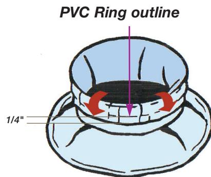
**Step 1.** Place the PVC Ring over the straight portion of the CBC Glove Extension.
