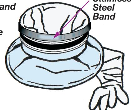
**Step 5.** Place the Stainless Steel Band directly over the Neoprene Band and tighten down.
